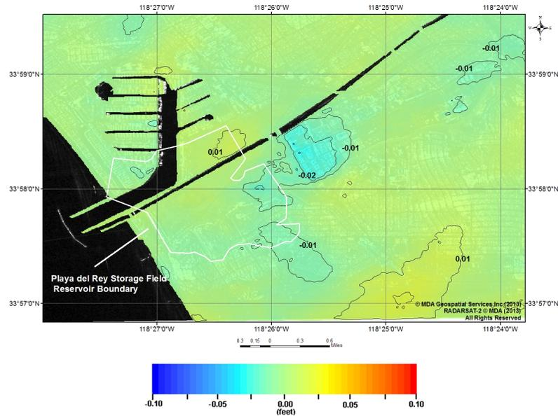
Figure 28: Vertical deformation from June 23, 2012 to September 3, 2012.
