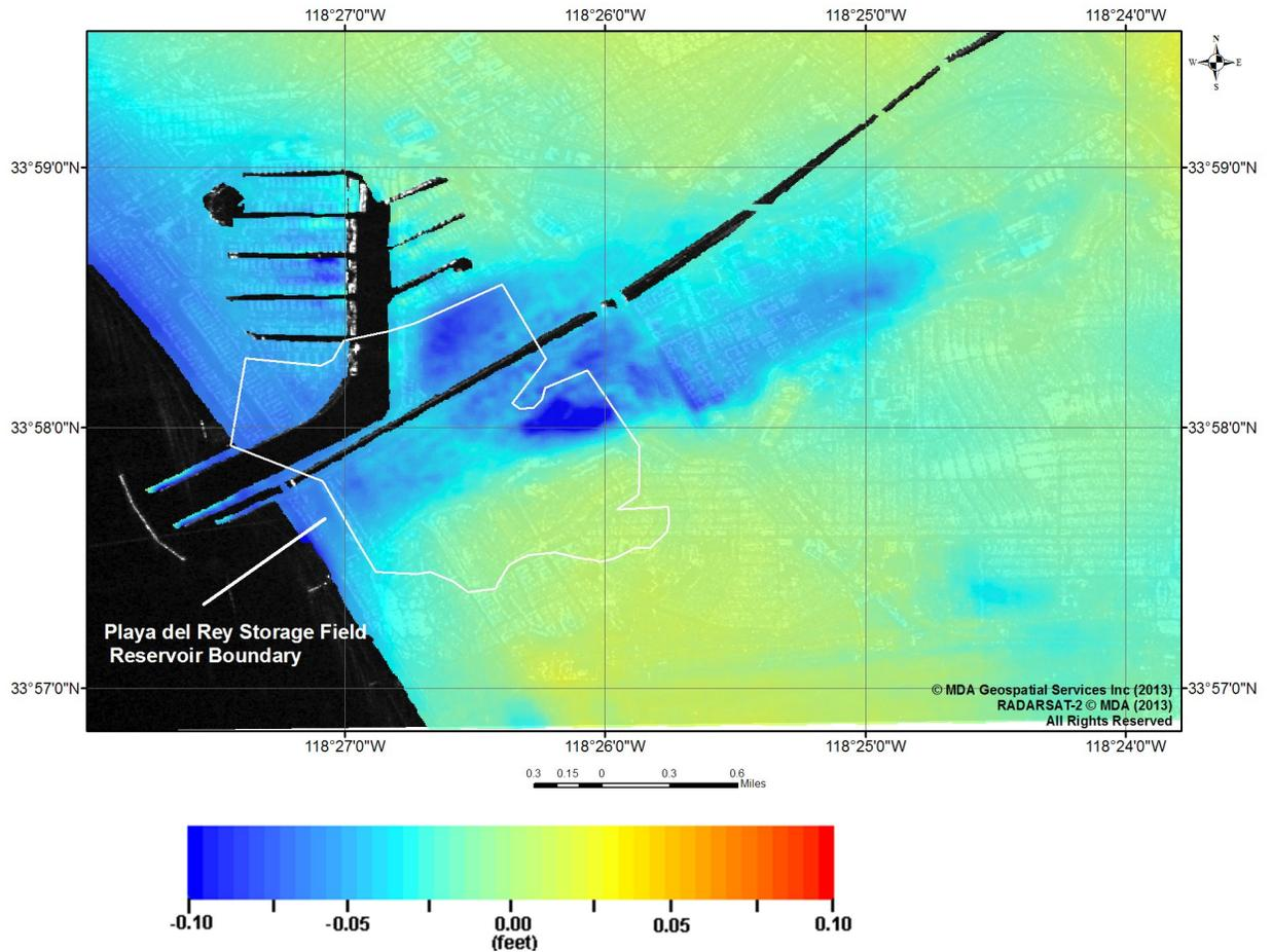
Figure 11: Playa del Rey Gas Storage Field AOI and surrounding area. Color representation of the cumulative vertical deformation from May 27, 2008 to June 18, 2013 superimposed onto SAR image.
