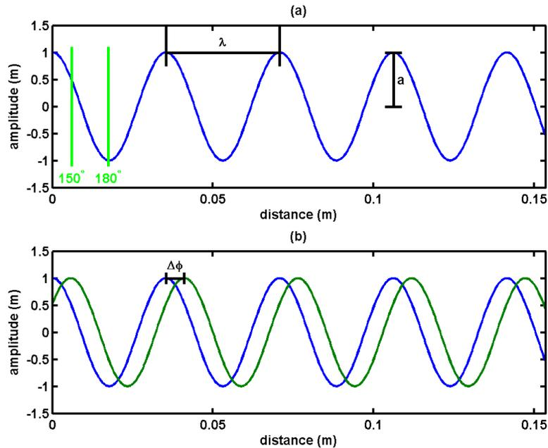
Figure 30: Definition of a 5.6-cm wave. Panel (a) shows the definition of wavelength,  $\lambda$ , and amplitude ( $a$ ). The green lines show the location on the wave associated with  $150^\circ$  and  $180^\circ$  of phase. Panel (b) demonstrates the phase difference,  $\Delta\phi$ , between two waves.
