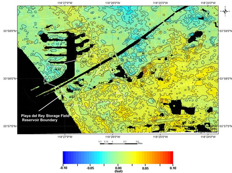
Figure 16: Vertical deformation from June 15, 2009 to September 19, 2009.
