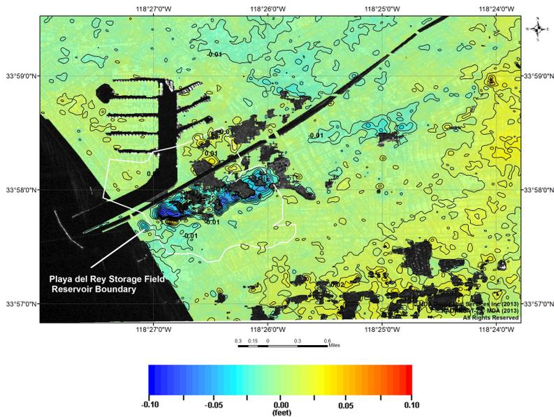
Figure 19: Vertical deformation from March 6, 2010 to June 10, 2010.
