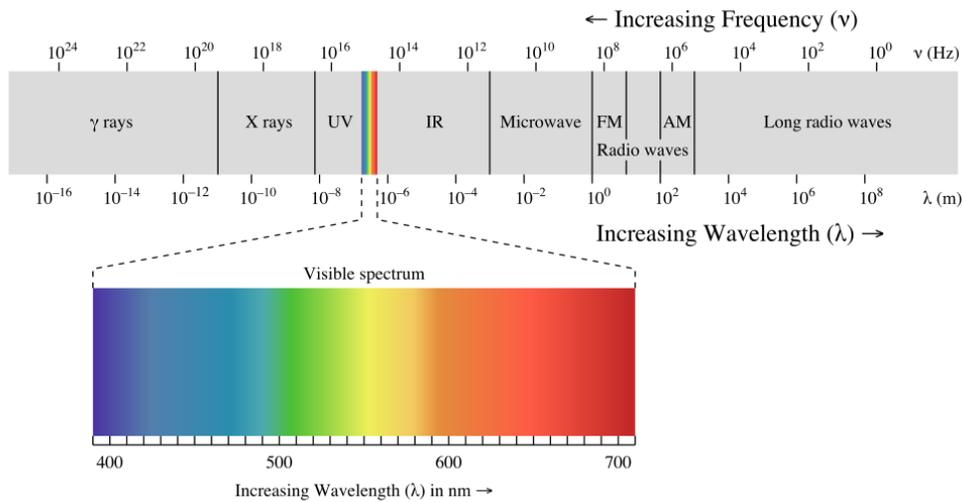
Figure 31: Electromagnetic spectrum showing the wavelength and frequency characteristics of radiation. The microwave portion of the spectrum contains the waves used for RADAR observation.
