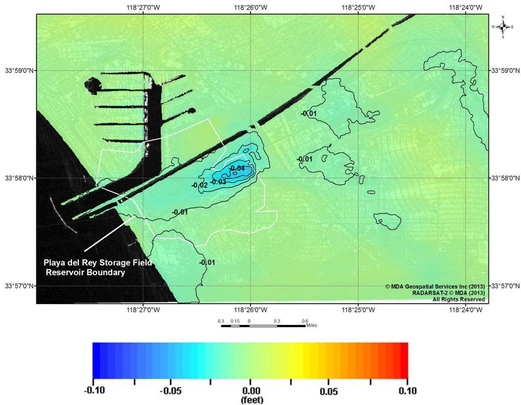
Figure 7: Zoom-in of Playa del Rey Gas Storage Field AOI and surrounding area. Cumulative vertical deformation from March 14, 2013 to June 18, 2013, with 0.01 ft contours.
