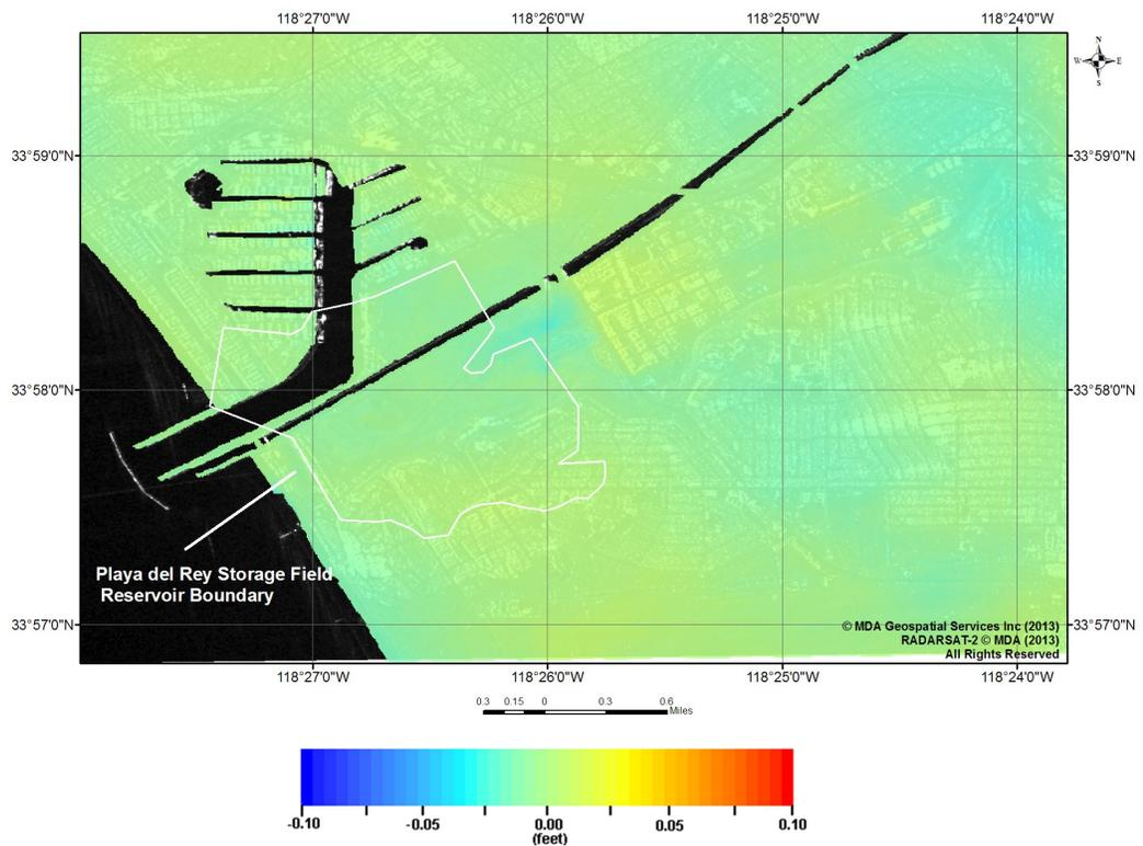
Figure 9: Zoom-in of Playa del Rey Gas Storage Field. Color representation of the summation of the vertical deformation products from December 8, 2012 to June 18, 2013 superimposed on SAR image with 0.01 ft contours. In this representation, blue corresponds to subsidence and red indicates uplift.
