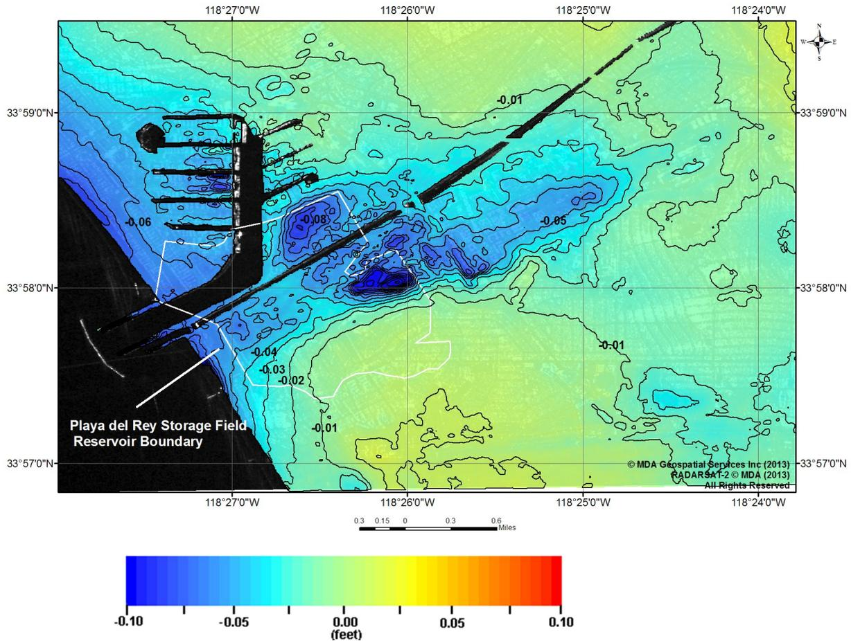
Figure 10: Zoom-in of Playa del Rey Gas Storage Field AOI and surrounding area. Cumulative vertical deformation from May 27, 2008 to June 18, 2013, with 0.01 ft contours.
