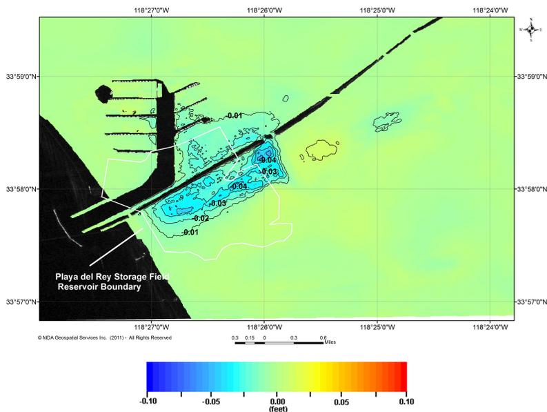
Figure 23: Vertical deformation from March 1, 2011 to June 29, 2011.
