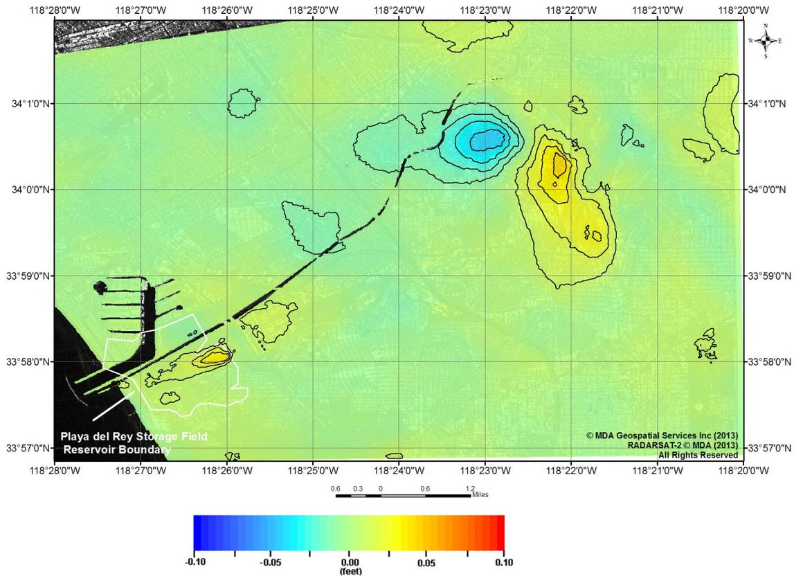
Figure 3: Playa del Rey Gas Storage Field AOI and surrounding area. Color representation of the vertical deformation product from December 8, 2012 to March 14, 2013 superimposed on SAR image with 0.01 ft contours. In this representation, blue corresponds to subsidence and red indicates uplift.
