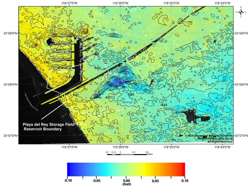
Figure 20: Vertical deformation from June 10, 2010 to September 14, 2010.
