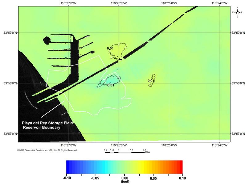
Figure 24: Vertical deformation from June 29, 2011 to September 9, 2011.
