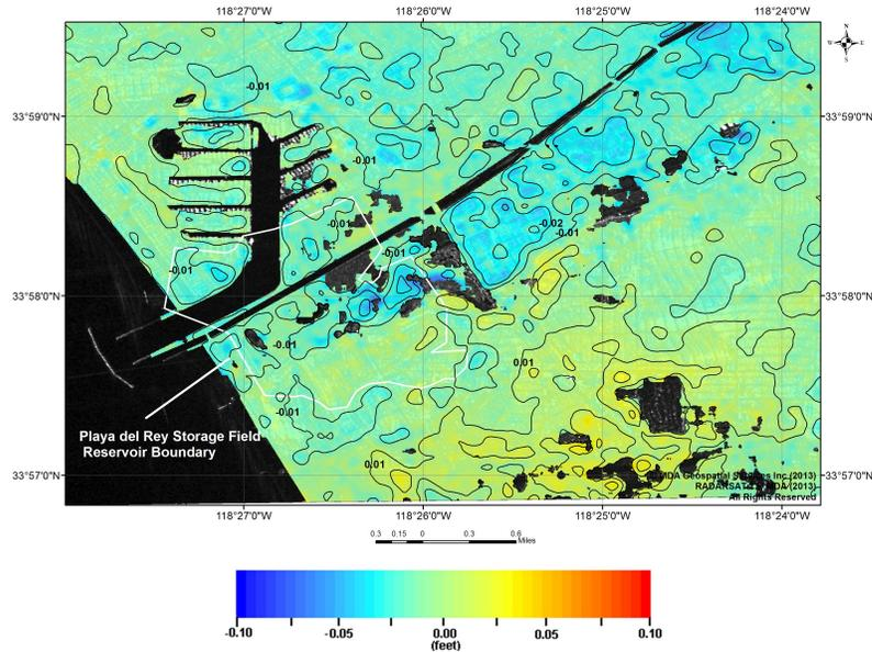
Figure 12: Vertical deformation from May 27, 2008 to August 31, 2008.
