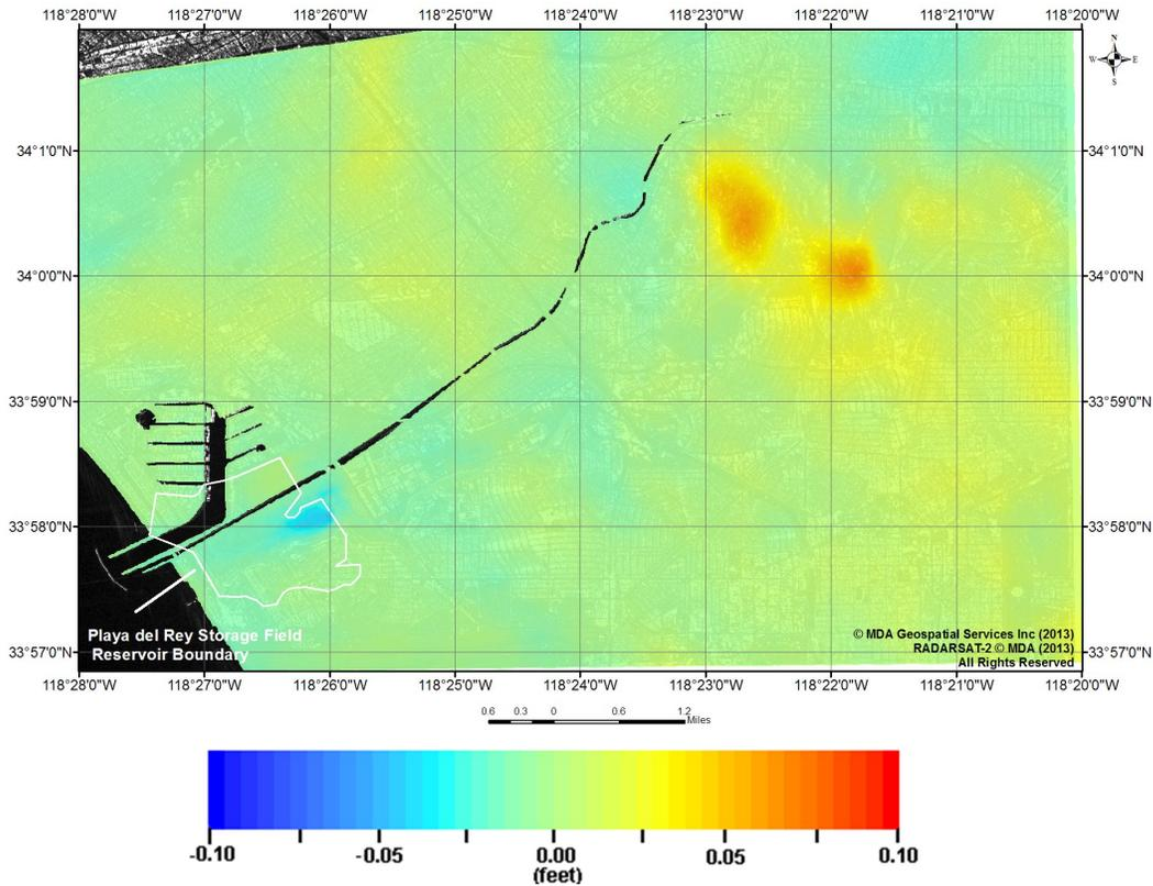
Figure 5: Playa del Rey Gas Storage Field AOI and surrounding area. Color representation of the vertical deformation product from March 14, 2013 to June 18, 2013 superimposed on SAR image without contours. In this representation, blue corresponds to subsidence and red indicates uplift.
