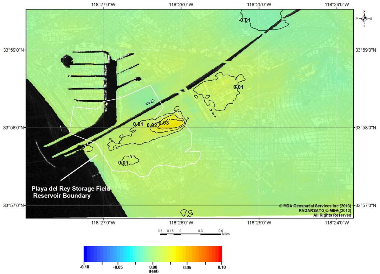
Figure 4: Zoom-in of Playa del Rey Gas Storage Field AOI. Color representation of the vertical deformation product from December 8, 2012 to March 14, 2013 superimposed on SAR image with 0.01 ft contours. In this representation, blue corresponds to subsidence and red indicates uplift.
