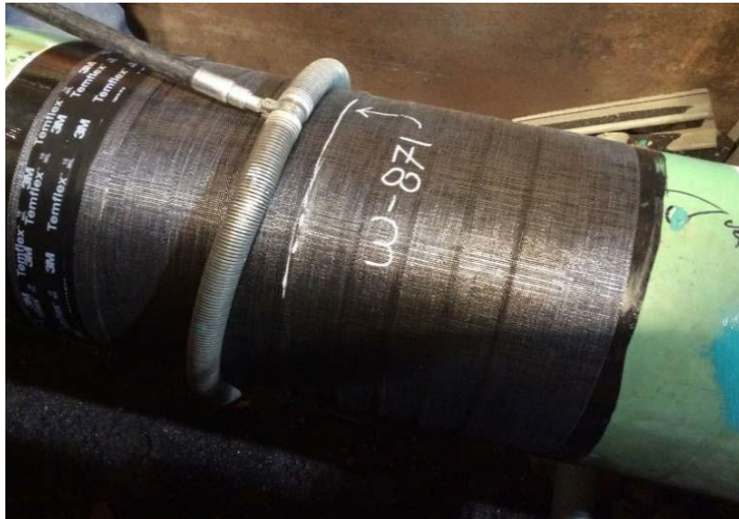
Figure 23: Electronic Inspection method - Holiday Testing of a Coated and Wrapped Weld
