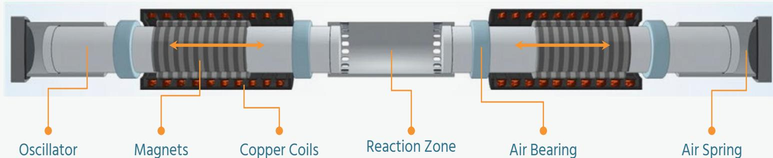
**The Linear Generator Core:** A linear generator is an electromechanical device that directly converts linear motion into electricity using chemical or thermal energy.
