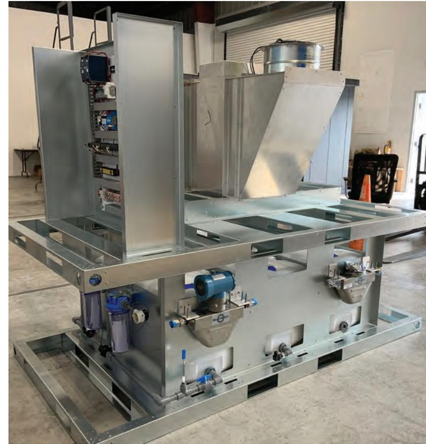
*The innovative A/C system incorporates heat recovered from gas-fueled CHP units—including fuel cells—via a load-shifting thermochemical energy-storage system that uses a liquid desiccant to store energy.*
