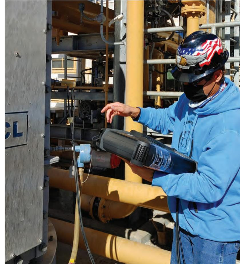
*To verify compliance with emission limits, plant and facility operators conduct expensive and complicated tests using EPA Reference Methods with analyzers in a large trailer or truck or handheld, electrochemical analyzers.*
