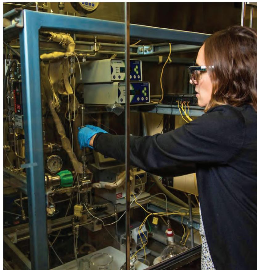
*A research team from PNNL and WVU developed and demonstrated a thermocatalytic decomposition process to convert methane into hydrogen at a bench scale. The process also yields a high-value solid carbon co-product suitable for a variety of manufacturing applications.*
