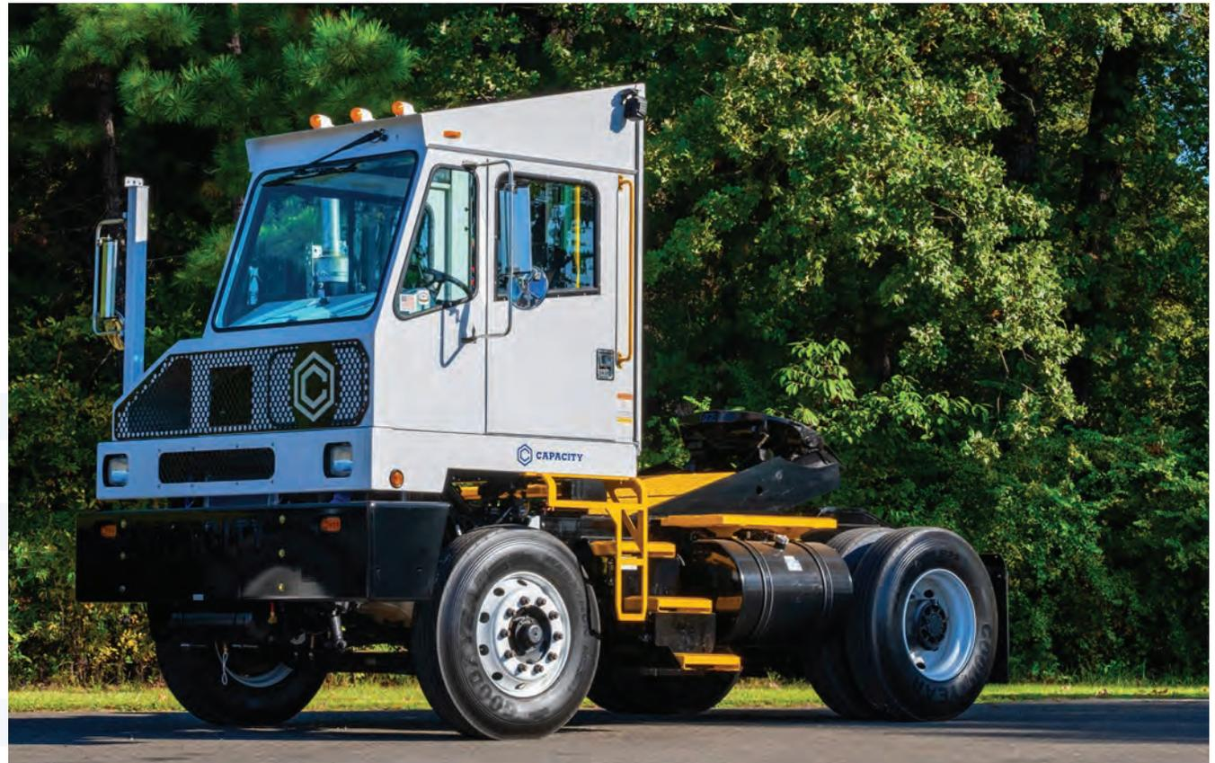
*The project team configured two diesel-powered Capacity Trailer Jockey Series TJ9000 gliders (above) with with an electric drive powertrain and a hydrogen fuel cell.*
